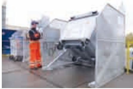
The containers are emptied by machine using lifting/tipping equipment which reduces the time needed to empty a bin by around 40 seconds. Furthermore, using electrically run equipment means the emptying process is much quieter.
